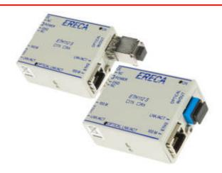
ERC ETH 112 module converts Ethernet 10/100 BASE-T (Standards IEEE 802.3 and IEEE 802.3u) to optical fiber 100 BASE-FX.
