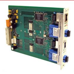
ERC ETH module converts Ethernet 10/100 BASE-T (Standards IEEE 802.3 and IEEE 802.3u) to optical fiber 100 BASE-FX.
