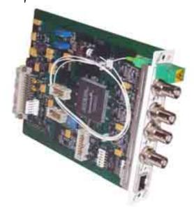
**ERC 4000** is bidirectional transmission equipment. It transmits 4 video, data and closure contact on one optical fiber.
