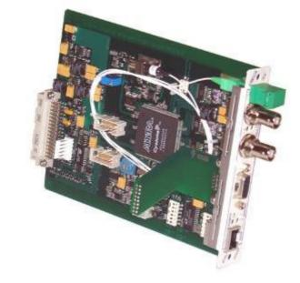
**ERC 2200** is bidirectional transmission equipment. It transmits 2 video, 2 audio, 1 serial data Channel and 1 contact closure on one optical fiber.
