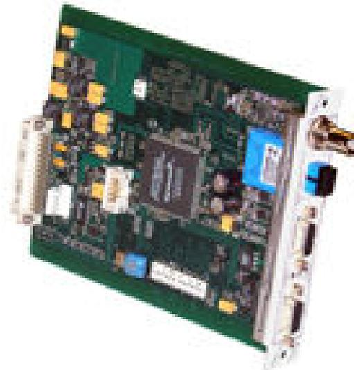
**ERC 1300** is bidirectional transmission equipment. It allows transmission of video signal, audio, data and contact closure on one optical fiber.
